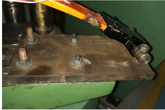
Fig 1 Fixture arrangement on UTM with fix end.
