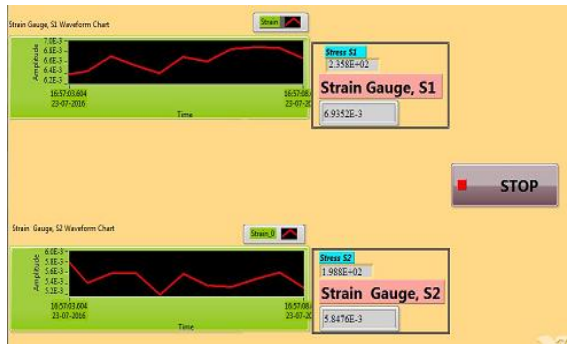
Fig. 4 Strain and strain measurement for 580N load
